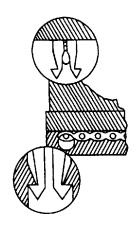
AMP-LATCH connectors have an additional feature not found in competitive connectors: Contact Latching. As the cable is terminated, a cover snaps down over the contacts.
