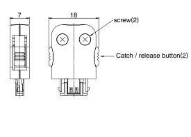
• 10 pos. (Reverse, shielded type, for 4mm max. cable diameter)
