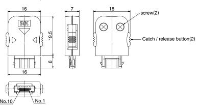
• 10 pos. (Reverse, non-shielded type, for 4mm max. cable diameter)
