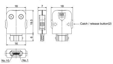
• 10 pos. (Shielded type, for 4mm max. cable diameter)
