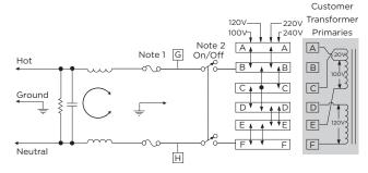
Note 1: Provision for dual Metric style fusing
