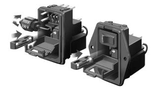
To change selected voltage: disconnect the power cord; open cover using a small blade screwdriver or similar tool; insert the tool into the voltage selection slot and remove wheel from unit; select desired voltage; replace wheel into unit and close cover, making sure the selected voltage appears in connector window.
