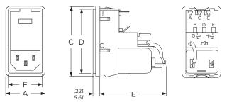
Non-switched model shown, for switched detail refer to flange models Metric fuse models have an additional jumper from filter to module
