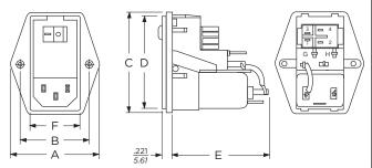
Switched model shown, for non-switched detail refer to snap-in models Metric fuse models have an additional jumper from filter to module
