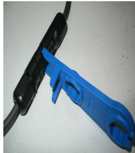
Separated by Wrench tool
