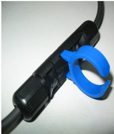
Separated by Ring tool
