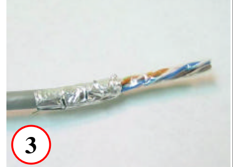
3 Fold back shield and drain wire
