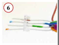
Slide trimmed Odd conductors into Odd row of Management Bar
