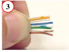
**Position Wires into Correct Configuration (586-B Shown)**
