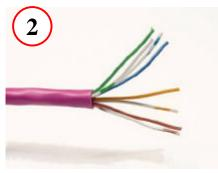
Untwist the pairs and Straighten the Wires
