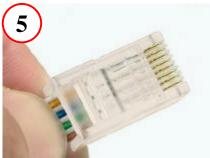
Insert Wires Along Plug Top, Maintaining Correct Alignment
