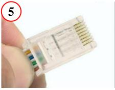
**Insert Wires Along Plug Top, Maintaining Correct Alignment**
