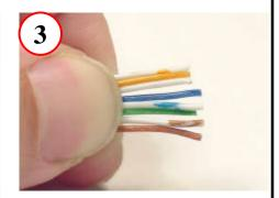
**Position Wires into Correct Configuration (586-B Shown)**
