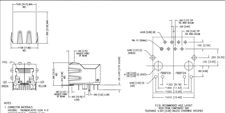
HOUSING: THERMOPLASTIC UL94 V-0
