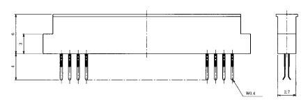
Recommended board thickness: 0.4 to 0.5mm
