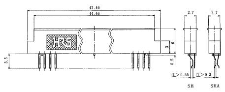
Recommended board thickness: 0.4 to 0.5mm
