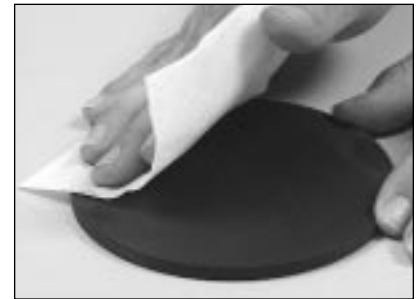
11.3 Clean the rubber pad with a lint free cloth moistened with isopropyl alcohol.
