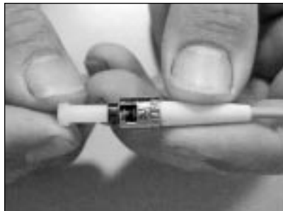
11.26 Install the dust cap on the connector.
