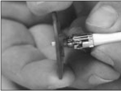
11.7 Place the connector ferrule in the polishing jig to verify that it fits properly. The fit should allow for easy movement of the ferrule.
