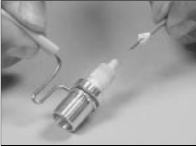
8.16 Gently insert the fiber into the connector.
