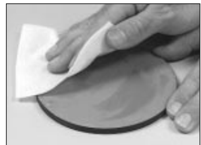
11.18 Clean the lapping film with a lint free cloth moistened with isopropyl alcohol.
