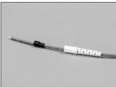
6.7 Place the strain relief boot and crimp ring on the cable.
