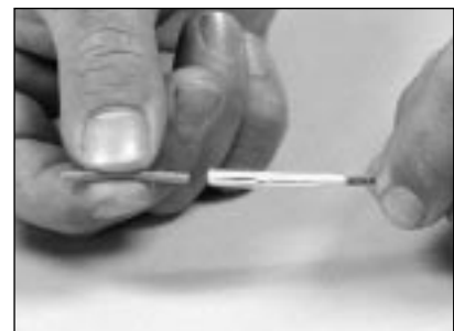
6.9 Remove the jacket from the end of the cable.
