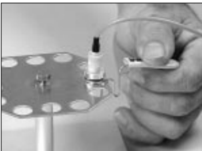
8.22 Place the connector holder into the cooling stand. The cooling time is about 3 minutes.
