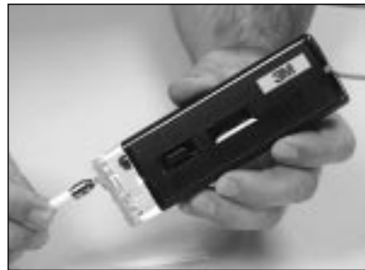
10.15 Inspect the connector end face with the view scope.
