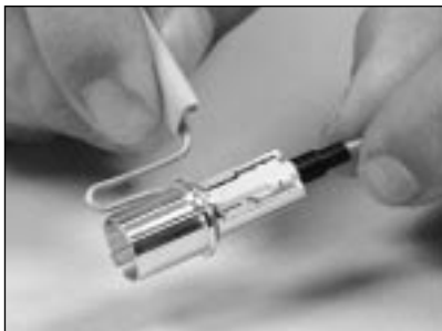
6.19 Slide the crimp ring over the aramid yarn until it is seated against the connector.
