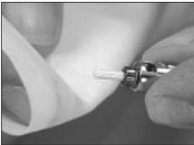
10.14 Clean the connector end face with a lint free cloth moistened with isopropyl alcohol.
