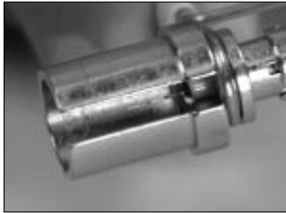
4.19 Bare fiber should be visible in the bottom of the connector holder.
