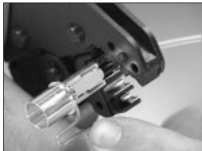
5.17 Crimp the larger part of the crimp ring with the .190 cavity of the crimp tool.
