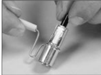
5.14 Slide the crimp ring over the backbone until it is against the connector.
