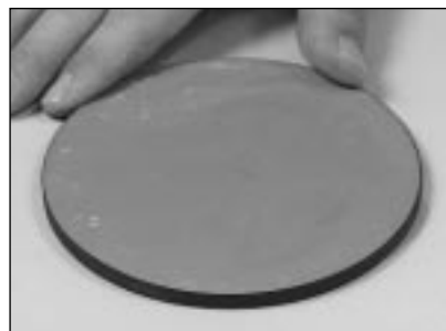
11.17 Before the alcohol evaporates, place the 0.05 Micron Lapping film (pale yellow) on the rubber pad shiny side down.
