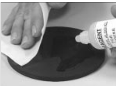
11.16 Wipe a layer of alcohol onto the rubber pad.
