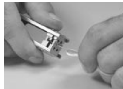
6.12 Remove the buffer in small pieces until \frac{1}{16} "– \frac{5}{8} " (14-16 mm) of the buffer remains.
