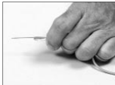
6.11 To prevent the buffered fiber from being pulled out, lace the cable through your fingers.
