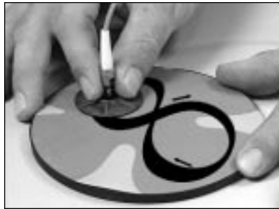
11.23 Polish the connector for 3 figure eights only.
