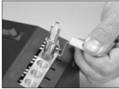
5.11 Remove the connector holder from the oven.
