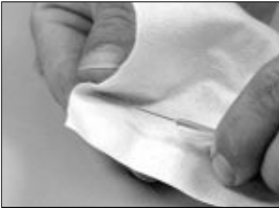
8.13 Clean the fiber with a lint free cloth moistened with isopropyl alcohol.
