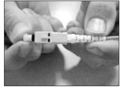
10.28 Install the dust cap on the connector.
