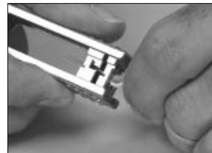
4.12 Remove \frac{5}{8} " (16 mm) of the buffer.
