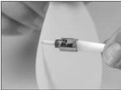
11.1 Perform an air polish on the fiber by gently moving the connector in a circular motion on the 2 micron lapping film (pale aqua color).
