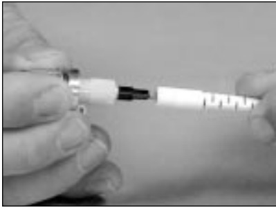
10.23 FC Connector—Install the boot on the connector.
