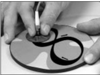
11.13 Beginning with a light pressure, move the jig in a figure eight pattern.
