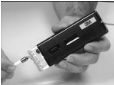
11.25 Inspect the connector end face with the view scope. Section 10 has pictures of properly and improperly polished connectors.
