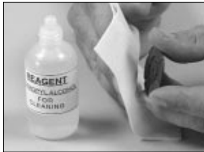
11.2 Clean the polishing jig with a lint free cloth moistened with isopropyl alcohol.
