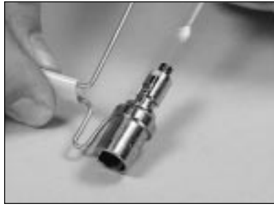
4.17 Gently insert the fiber into the connector.
