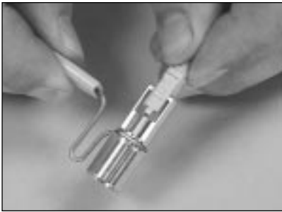
6.4 Load the connector into the SC connector holder.
