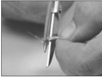
8.14 Cut the aramid yarn to \frac{5}{16} " (8 mm) long.
