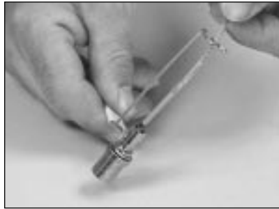
4.20 Secure the cable to the cable holder.
