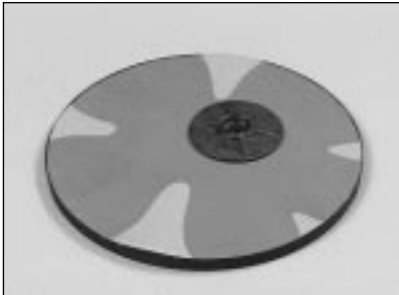
11.10 Place the jig on the lapping film.
