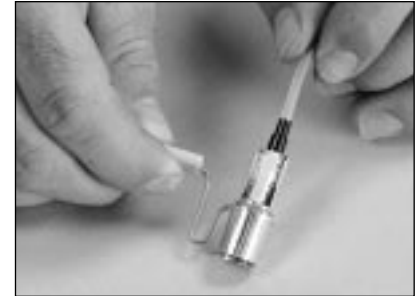
5.15 Slide the clear strain relief tube into the crimp ring.
