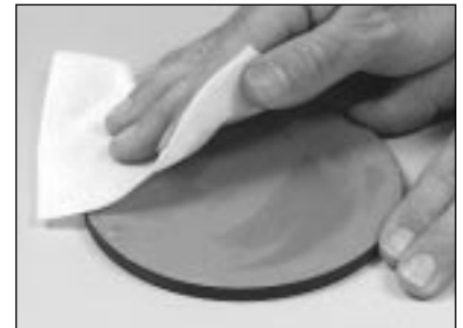
11.6 Clean the lapping film with a lint free cloth moistened with isopropyl alcohol.
