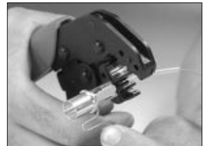
5.18 Crimp the smaller part of the crimp ring using the .137 cavity.
