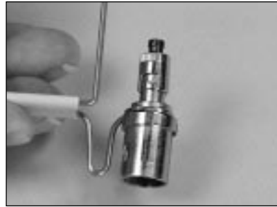
4.5 Latch the connector bayonet housing to the connector holder.
