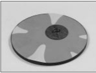
10.10 Place the jig on the lapping film.
