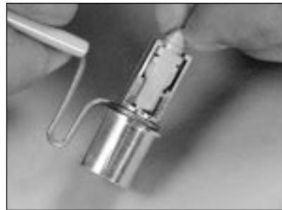
5.5 Push down on the connector and turn it 90 degrees so that the arms hold the connector in place.
