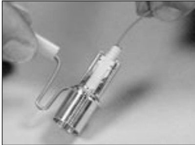
5.13 Push the buffered fiber until it stops.
