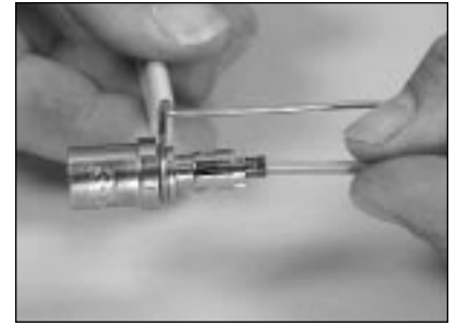
4.18 Push the cable until the aramid yarn is inside the connector.
