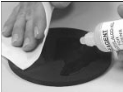
11.4 Wipe a layer of alcohol onto the rubber pad.
