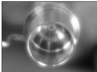
6.20 Verify that the bare fiber is visible in the bottom of the connector holder.
