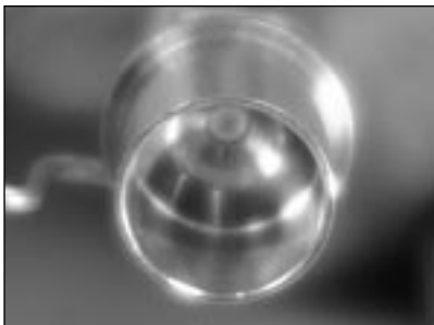
5.16 Verify that the bare fiber is visible in the bottom of the connector holder.
