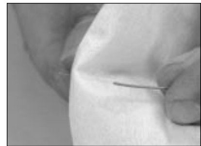
7.9 Clean the fiber with a lint free cloth moistened with isopropyl alcohol.
