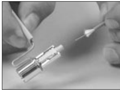
6.17 Gently insert the fiber into the connector.
