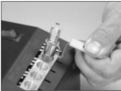
6.16 Remove the connector holder from the oven.
