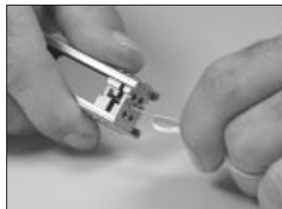
8.11 Remove the buffer in small pieces until \frac{1}{16} " (14 mm) of the buffer remains.
