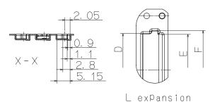
Emboss taping specification (Based on taping of electronic parts [JIS 0806])
