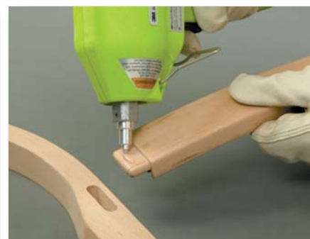
Adhesives are available for bonding a variety of wood sizes and configurations such as this mortise and tenon assembly.
