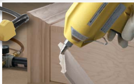
With a thin bond line, PUR 250 adhesive makes a secure, aesthetically-pleasing crown molding assembly.
