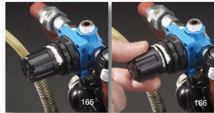
To indicate that a valve setting is not to be changed and to know if it has, 3M™ Scotch-Seal™ Tamper-indicating Sealant 1252 clearly communicates before and after tampering.
