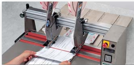
241 A variety of automatic and semi-automatic equipment is available for higher volume applications. For example, apply tape to business forms, literature, bounce back and business reply cards.
