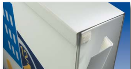
Die-cut 3M™ Scotchmate™ Reclosable Fasteners secure metal edge molding around an internally-illuminated sign. The molding holds the sign face in place and is readily removed for bulb replacement. 289
