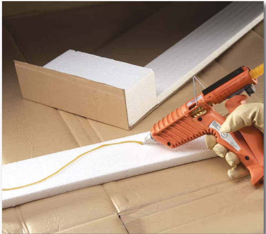
3M™ Scotch-Weld™ Hot Melt Applicator LT with 3M low temperature (265°F/129°C) adhesive effectively bonds heat-sensitive substrates such as styrene foam to itself, corrugated, or other surfaces without damaging the foam.
