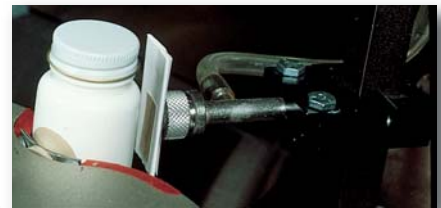
242 3M™ Extended Liner Tapes 450XL, 450EK and 465XL immediately bond product information “outserts” to polyethylene bottles. Holds tightly but can be cleanly removed.
