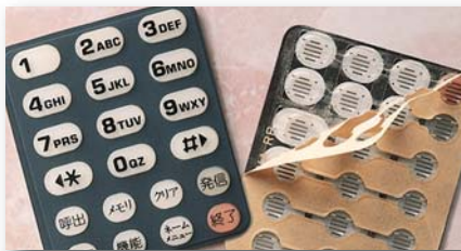
With differential adhesive, the silicone adhesive side of 3M™ Double Coated Tape adheres to a silicone rubber keypad. Acrylic adhesive side adheres to a plastic base.
