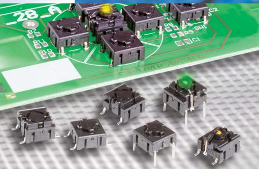
The Multimec 5E and 5G series is the new generation of the existing 3A, 3C, 3E, 3F, 4A and 4Fmultimec switches. The 5E and 5G series is a narrower product line, but the flexibility is more advanced. The switches will be supplied in high temperature material only to stand today's advanced soldering processes. The cap holding system is improved, by a superior snap system.
