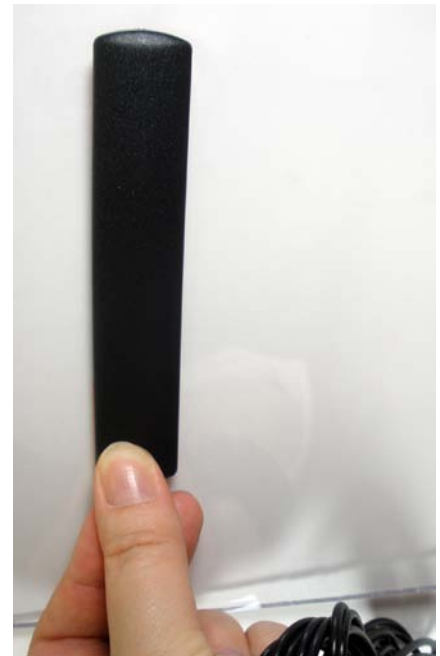
Figure 18. Adhesive Mount Antenna – Step 3. Mount the Antenna
