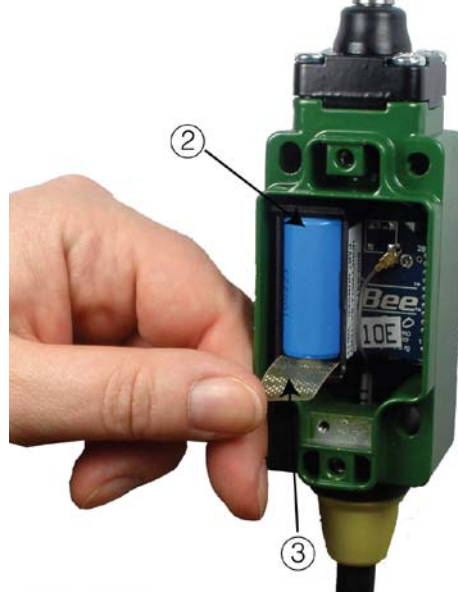
Figure 3. Limitless™ Battery and Insulator
