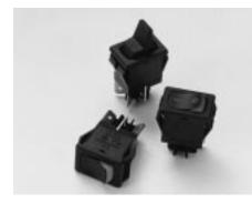
The miniature 611/621-Series switches are double insulated and available in single or double pole. These snap-in mounting style switches are available with paddle, rocker or Visi-Rocker type actuators. A variety of terminations are offered with ratings through 11 amps. International approvals are also available.
