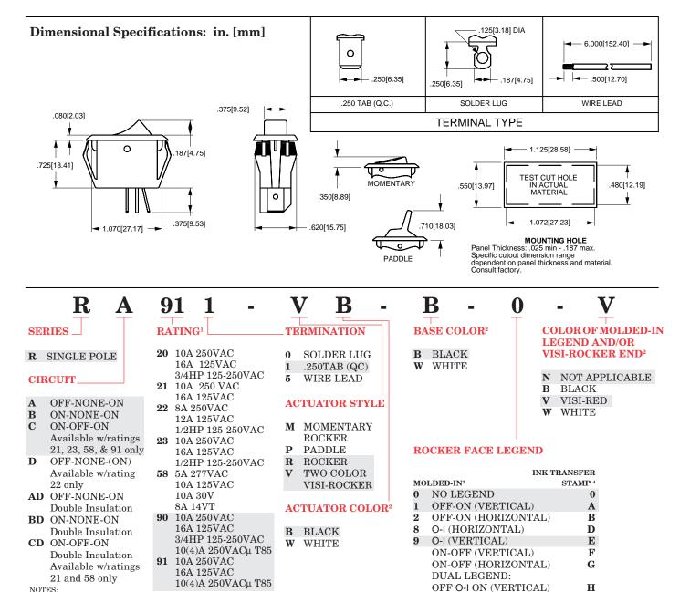
Shading indicates standard configurations.
