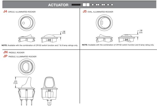
NOTE: JP actuator available with the of CR102 switch function and 7 & 8 lamp ratings only
