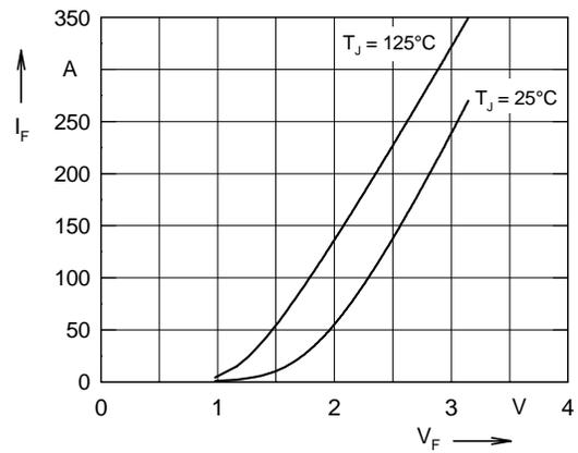
Fig. 4 Typ. forward characteristics of free wheeling diode
