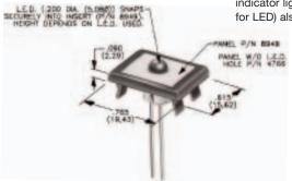
Above frames (part nos. 432XXXXXX) are also available with insert which accepts LED for indicator light assembly. Order insert separately from frame. Blank insert panel (without hole for LED) also available. **LED not included.**
