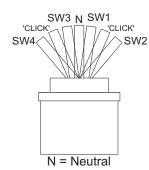
As per option D, but with a mechanical detent between actuation of the first and second switch.
