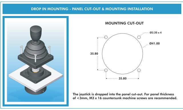
Note: The dimensions shown are for a generic 8000 Series with the conical E type handle. For specific dimensions of this or any other configuration please refer to Apem.
