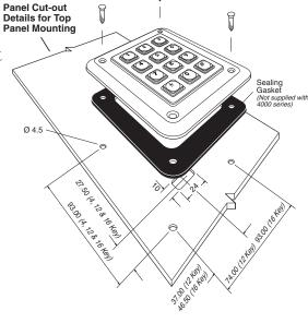
Countersunk Fixing Screws (Not Supplied) (Threads must be sealed to prevent water ingress)
