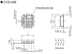
Unless otherwise specified, tolerance :  $\pm$  0.3 (Unit : mm)
