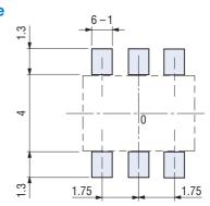
Note) The zero point is the center of mounting.
