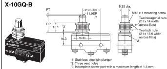
Note: Do not use both the M12 mounting screw and the mounting holes in the case at the same time. Doing so will cause stress to be applied to the Switch, possibly damaging the case or cover.
