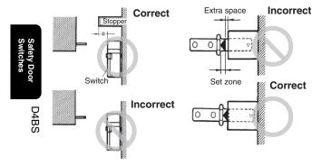
Refer to *Dimensions* for the mounting dimensions of the Operation Key and mount the Operation Key correctly. The Operation Key will soon become damaged or worn out if it is not mounted correctly.
