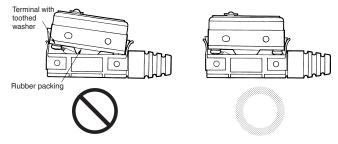
• Use round solderless terminals having the following dimensions to connect leads to the terminals. Tighten the screws of terminals to a torque of 0.78 to 1.18 N·m. Use the terminal shown below.
