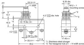
. Stainless-steel plunger . Two hexagonal nuts (2 t  $\times$  14 width across flats) . Two lock nuts (2 t  $\times$  15.6 width across flats) . Incomplete screw part with a maximum length of 1.5 mm.
