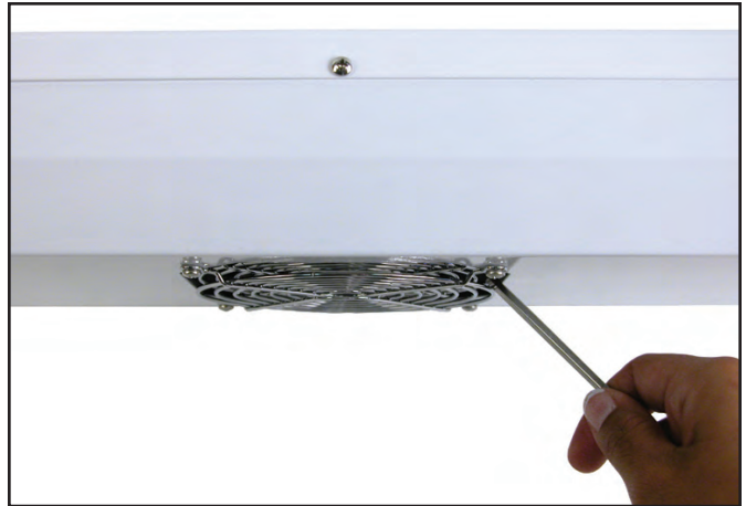
Figure 8. Shorting the ionizer's two fan grills
