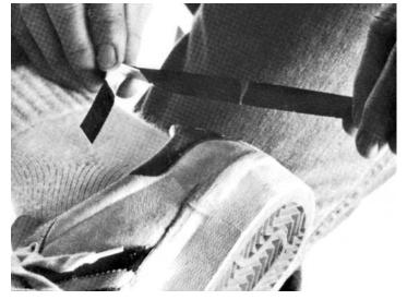
3. Bend metal clip to fit over edge of shoe.
