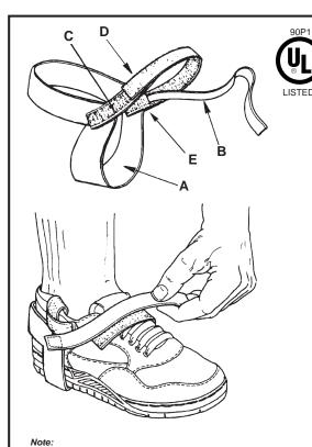
Two heel straps are recommended for reliable grounding and ESD
