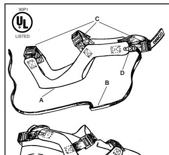
Two heel straps are recommended for reliable grounding and ESD protection, providing ground when one foot is off the floor.
