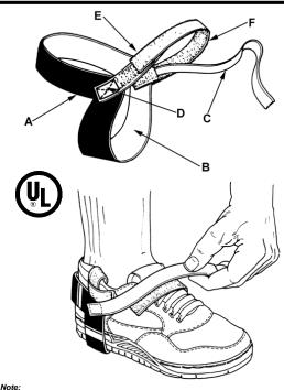
"ESD protective footwear is designed to reduce body charge levels by supplying a conductive path from the body to the floor material. Heel and toe grounders shall be worn on both feet to insure effective use
