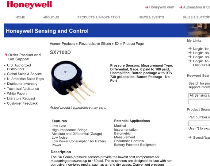
measuring pressures up to 150 psi. These sensors are designed for use with noncorrosive, non-ionic media, such as air and dry gases. Convenient pressure ranges are available to measure differential, gauge, and absolute pressures from 0 psi to 1 psi (SX01) up to 0 psi to 150 psi (SX150).
