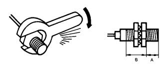
Do not exceed the torque listed in the table below when tightening the mounting nuts.
