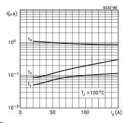
Switching Times Inductive Load Versus Temperature
