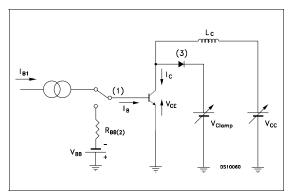
(1) Fast electronic switch(3) Fast recovery rectifier
