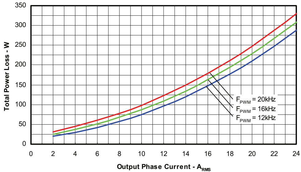
Figure 6. Total Power Losses vs. Output Phase Current Sinusoidal Modulation, V^+ = 100V , T_j = 150^\circ C , Modulation Depth=0.8, PF=0.6
