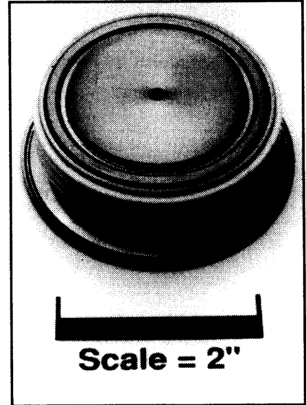
R9G2_12 Fast Recovery Rectifier 1200 Amperes Average, 3600 Volts
