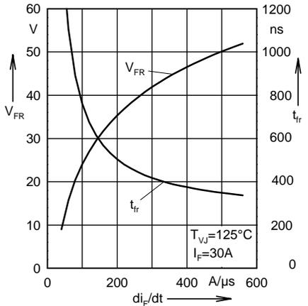
Fig. 6 Peak forward voltage versus  $di_F/dt$ .
