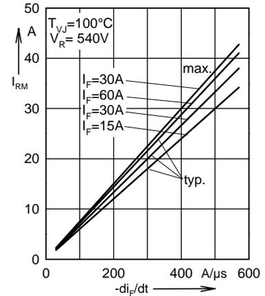
Fig. 3 Peak reverse current versus  $-di_F/dt$ .
