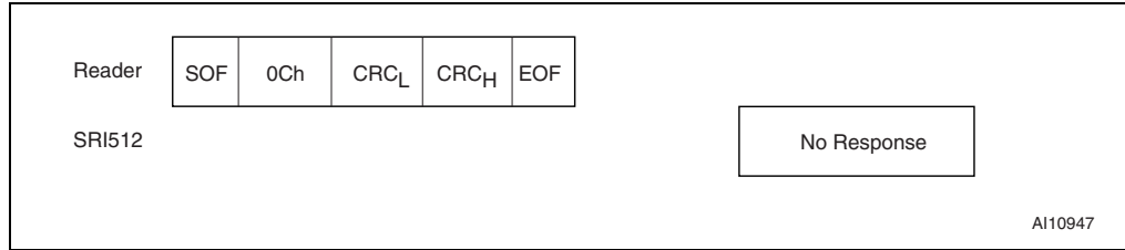
Figure 58. Read_block frame exchange between reader and SRI512
