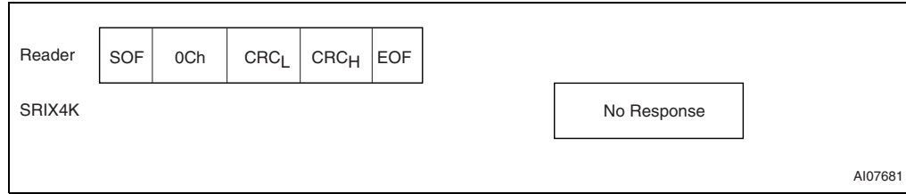
Figure 59. Read_block frame exchange between reader and SRIX4K
