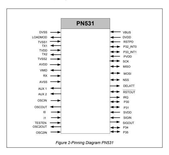
The device operates with six individual power supplies for best performance in terms of EMC behaviour and signal de-coupling. This gives outstanding RF performance and maximum flexibility to adapt to different operating voltages of digital and analog parts.
