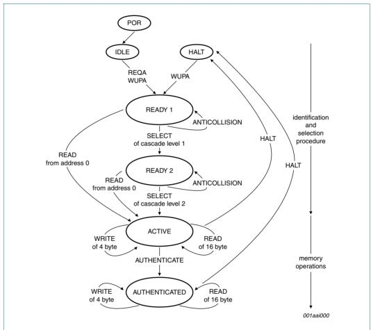
**Remark:** Not shown in this diagram: In each state the command interpreter returns to the Idle state if an unexpected command is received. If the IC has already been in the Halt state before it returns to the Halt state in such a case.
