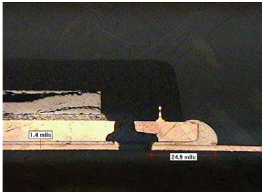
37% Paste Coverage, Plugged Via, 1.4 mil Standoff
