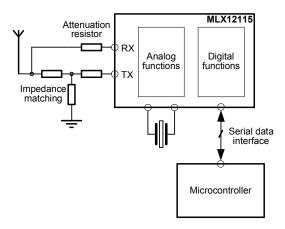
The main features include user selectable modulation depth in write mode, whereas single sub-carrier ASK and FSK modulations are recognized in the read mode.
