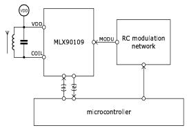
(1): MODE/SPEED config settings (2): DATA/CLOCK outputs
