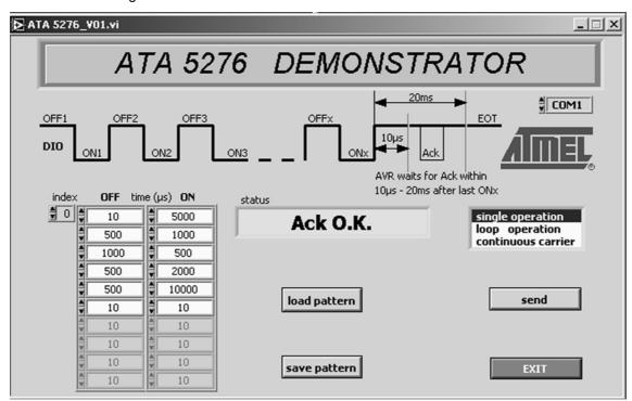
Figure 3-1. Command Settings on the Host Screen
