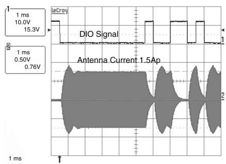
Figure 6-7. Antenna Current in Regulation
