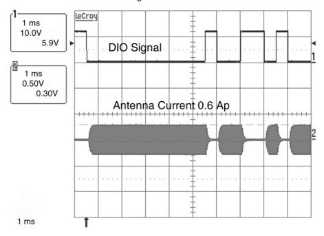
To reach the current regulation level of 1.5 Ap (see Figure 6-7), the series resistor RANT (R1) on the antenna module has to be shorted. In this case, the antenna quality factor is increased to Q = 108. Due to the high Q-factor, the current regulation leads to a short overswing during the switch-on phase. In the shorted R1 state, the antenna can also be operated with half current 0.75 Ap by opening jumper J3 (RCR = RCR1 =  $100 \text{ k}\Omega$ ).
