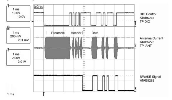
Figure 6-9. Signal Transmission ATAB5276 Transmitter to ATAB5282 Receiver
