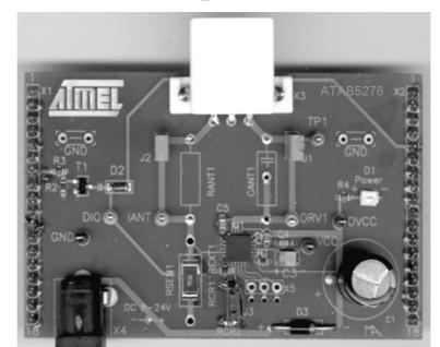
Figure 4-1. Transmitter Board ATAB5276\_V1
