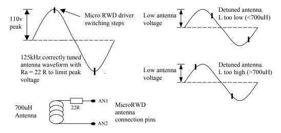
6) For optimum performance the antenna Q should not exceed 20 and to achieve reliable tuning at 125kHz the antenna inductance should be around 700uH. Higher Q and inductance values will still function but with a reduced range and performance.
