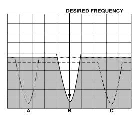
Antenna resonance should not be confused with antenna impedance. The difference between resonance and impedance is most easily understood by considering the value of VSWR at its lowest point. The lowest point of VSWR indicates the antenna is resonant, but the value of that low point is determined by the quality of the match between the antenna, the transmission line, and the device to which it is attached.
