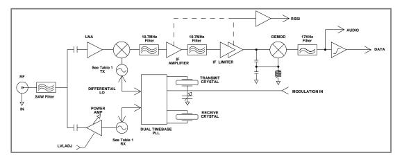
Figure 6: SC Series Block Diagram
