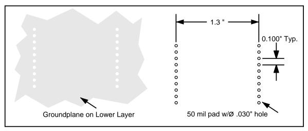
Figure 8: Recommended PCB layout
