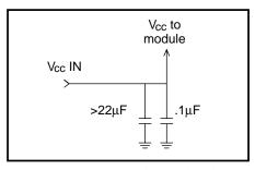
volts DC. The module's power-supply line should have bypass capacitors configured as shown in figure 7. Actual capacitor values will vary depending on noise conditions.
