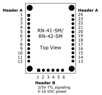
Signals on **Header A** except pins 4, 5, 6 and 7 have the following logic levels.
