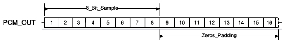
A 16-bit slot with 8-bit companded sample and zeros padding selected
